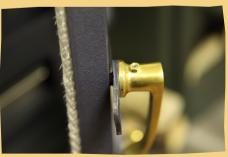
You will notice the door handle is on a thread. A simple turn either clockwise or anti clockwise will make the handle easier or harder to close, but use the card to make sure the rope gasket is holding tight. This way you control air supply, and ultimately the fuel consumption of the stove.
