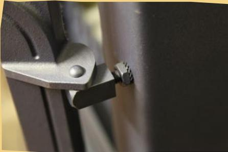
The door is hung on two hinge blocks. Simply lift the door off, like a garden gate and set to one side. The hinge blocks can now be turned clockwise, by 180 degrees, or half a turn. Hang the door again, close it on the card and make sure it is holding tight. If it is, you can move on to the handle.
