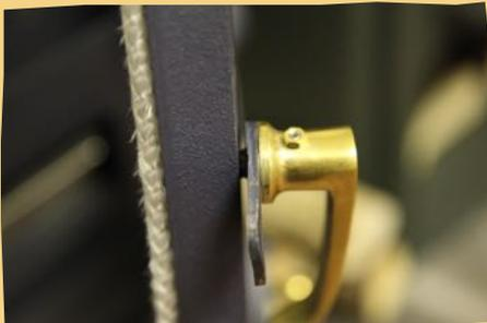
You will notice the door handle is on a thread. A simple turn either clockwise or anti clockwise will make the handle easier or harder to close, but use the card to make sure the rope gasket is holding tight. This way you control air supply, and ultimately the fuel consumption of the stove.
